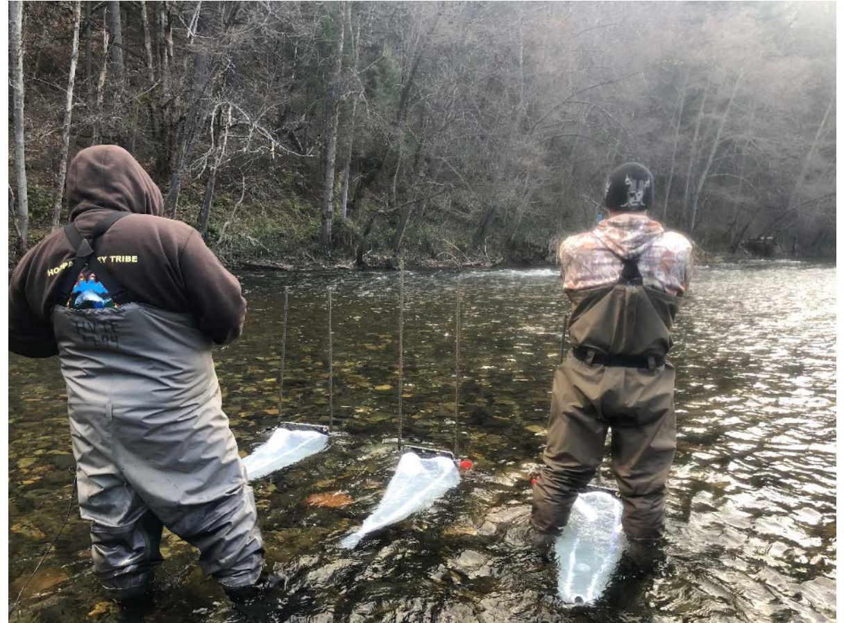
Temp, dissolved oxygen, and flow measured in front of each drift net on the Trinity river at Steel Bridge. Apr. 2018. Photo by Thomas S-O.
