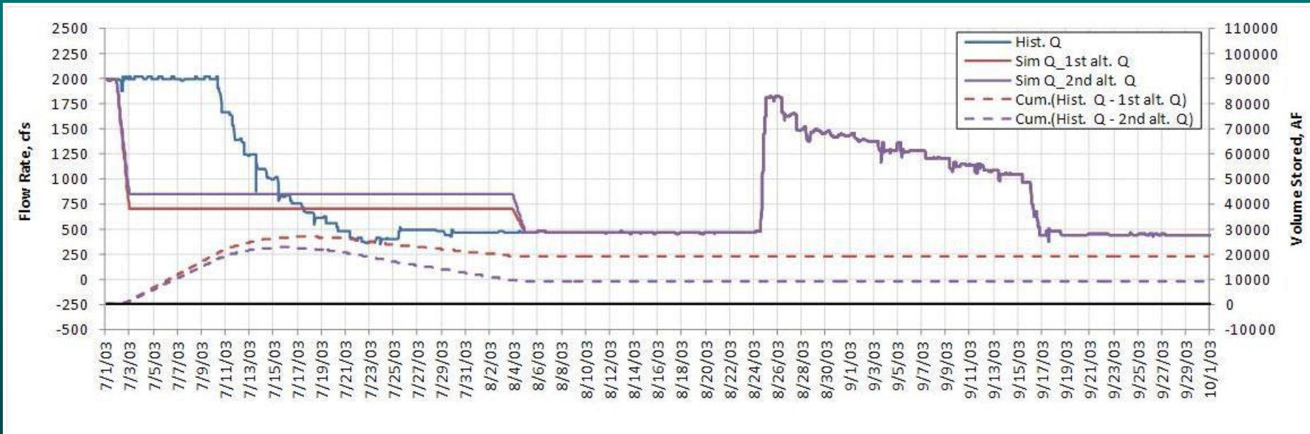
Figure 23. Scenarios with the alternative flow regimes. Historic flow rate vs. alternative flow rates, volumes stored. Year 2003.
