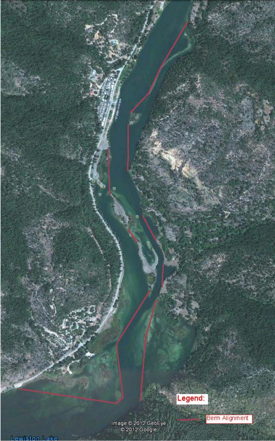
Figure 6. Dredging & Berm Alignment.
