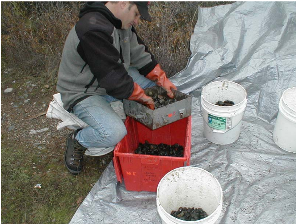
Figure 6. Initial wet sieving of bulk sample through 16 mm screen in rocker box.
