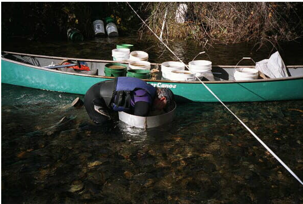
Figure 5. Bulk sampling using modified 2' diameter McNiel type sampler. Canoe was used to retain buckets during sampling and transport to the bank for sieving.
