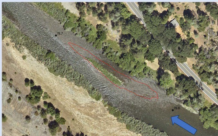
Erosion and inundation of a coarse, active bar observed in 2014 to a relatively small, vegetated island in 2023 between RMs 78.7 and 78.8
