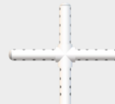
Figure 8. Schematic of the flow diffuser, which is installed at the bottom of the egg/incubation tank
