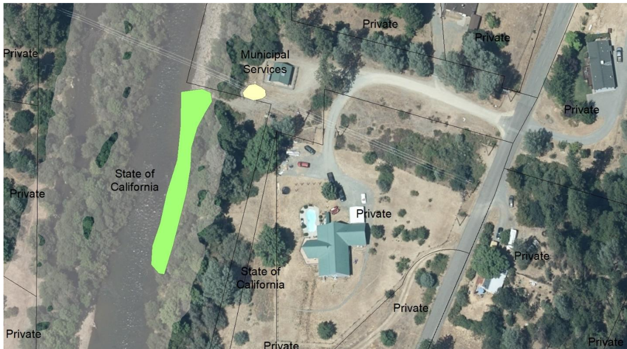
FIGURE 6. Gravel dump (yellow polygon) and placement area (green polygon) at Cableway. The shaded area in the channel is 1,050 cfs modeled on the 2016 topography by Bradley (2018). Approximate property boundaries are shown and parcel ownership type are labeled.
