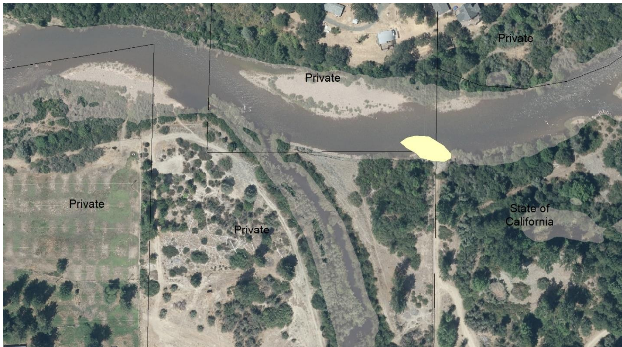
FIGURE 7. Gravel augmentation location at Fenceline on Lowden Ranch (yellow polygon). The shaded area in the channel is 4,000 cfs modeled on the 2016 topography by Bradley (2018). Approximate property boundaries are shown and parcel ownership type are labeled.
