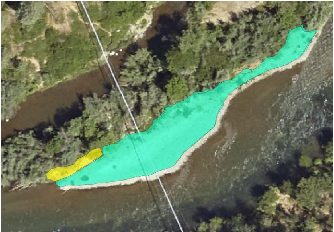
Figure 3. Repeat measurements of a large coarse bar (green) and a small fine sediment deposit (yellow) made on September 18 at RM 110.0. The difference in area between the fine deposit measurements was 26.2% and the coarse bar areas differed by 0.2%. The fine sediment deposit shown here is the upstream-most deposit of fines in the restoration reach. The aerial photography pictured is from July 12, 2023 when the daily average flow at Lewiston Dam was 456 cfs.
