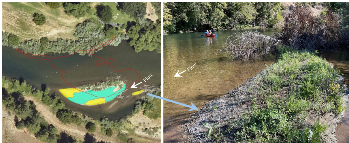
Figure 2. Coarse and fine sediment deposits mapped at RM 83.6 on the Trinity River in summer 2023 (left panel). The green area is a coarse bar and the yellow areas are fine sediment deposits. The coarse bar mapped here in 2014 is outlined in red. The right panel is an upstream view of a fine sediment deposit.
