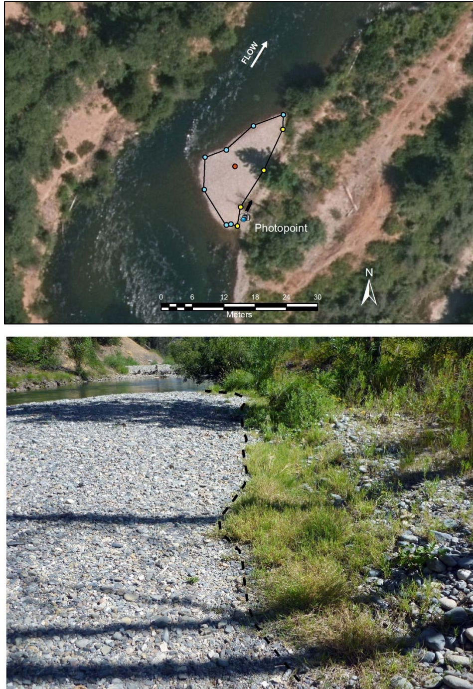
Figure 2. Top photograph: Example mapping polygon (black line) showing GPS points delineating boundaries of the active bar surface. Yellow dots show terrestrial contacts, blue dots show water contacts, and red dot shows bar centroid. Photographs were taken at each bar to show the back-bar contact that separates mobile from immobile areas; camera icon at upstream end of the bar shows the location and aspect of this photograph. Bar location is 4.27 km (2.65 miles) downstream of Lewiston Dam in Subreach 3 (bar centroid ID number 100), within the limits of the Sawmill channel rehabilitation site. Bottom photograph: back-bar contact separating the mobile from immobile area (shown by dashed black line). View is from upstream end of the bar facing downstream, photograph location and aspect arrow are shown in the top photograph.
