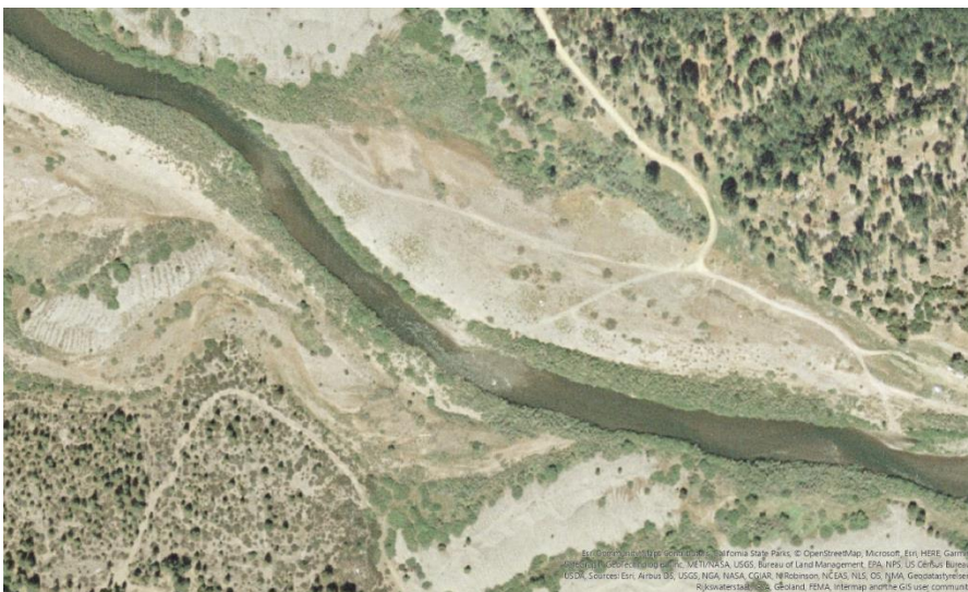
Aerial imagery collected by the U.S. Bureau of Land Management of the Chapman Ranch area in 1980. After construction of Trinity and Lewiston Dams which led to channel simplification.
