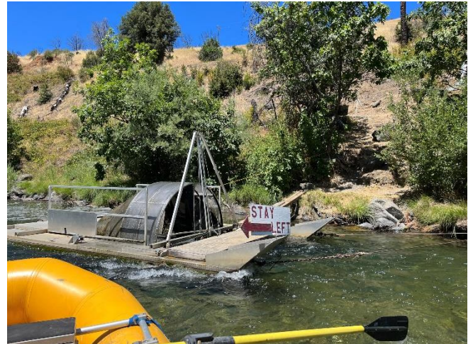
A Yurok Tribal Fisheries Department fish screw trap station. (Yurok Tribal Fisheries Department)
