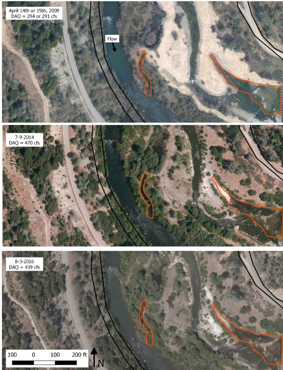
Figure 19. Aerial photographs showing two alcoves at the Sven Olbertson site constructed in 2008. The most successful alcove at this site, and one of the oldest functioning alcoves on the river, is shown in the center of each photograph. The GCD analysis and aerial photographs suggest that there has been no deposition in this alcove through time. This alcove is unique compared to others because it is surrounded by thick vegetation on all sides. The lack of sediment supply upstream of the alcove, the narrow mainstem channel width, and dense vegetation on the banks is likely why it has not aggraded. The Sven Olbertson site is the first downstream of the dam, so sediment input is limited. The reported flows are from the USGS Trinity River at Lewiston gage (gage # 11525500).
