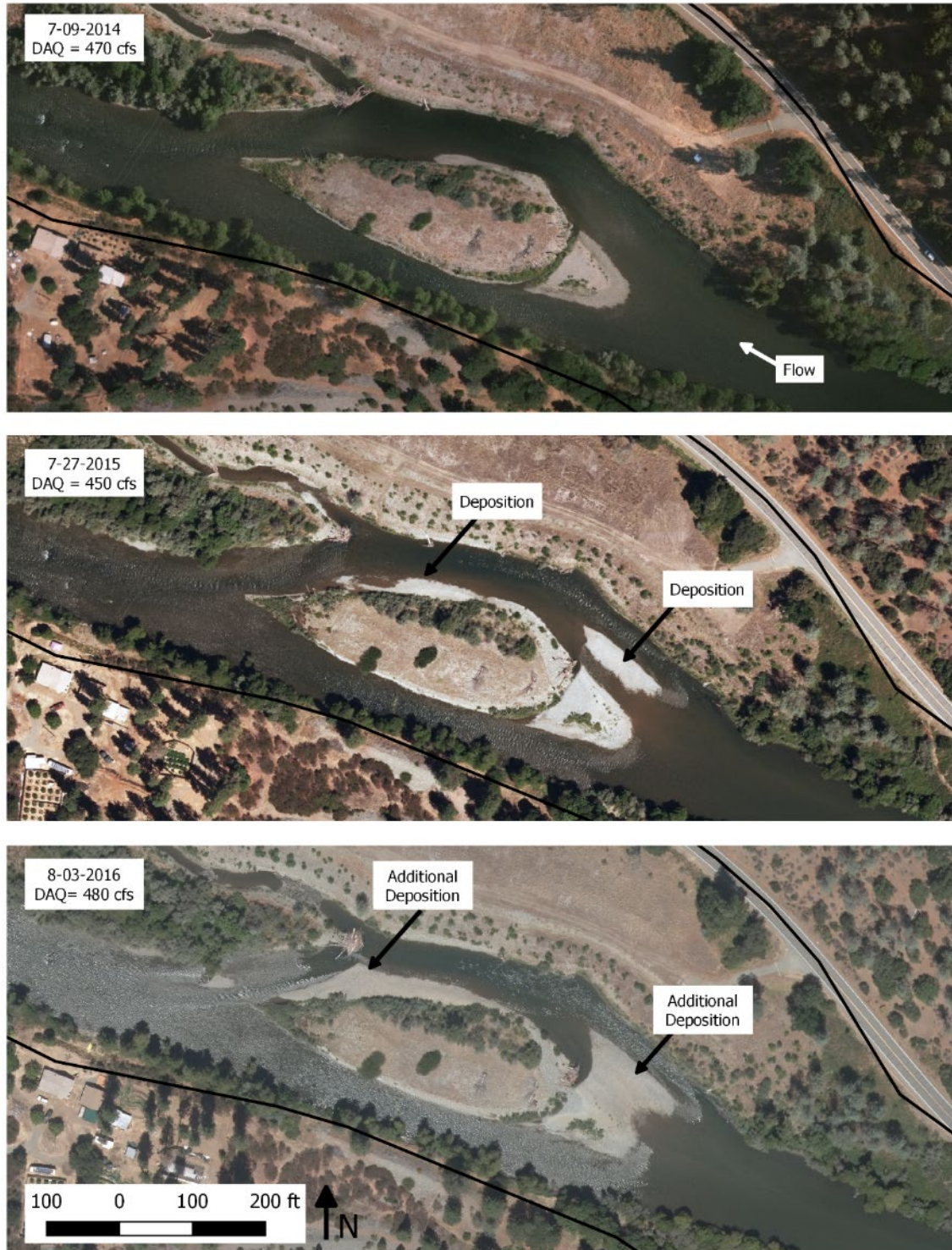
Figure 11. Aerial photographs from 2014–2016 that show deposition occurring through time in the split-flow channel at Wheel Gulch, constructed in 2011. The 2014 aerial photo is shown instead of the 2011 aerial photo because no noticeable change occurred between 2011 and 2014, and the 2014 image is of better quality. Note that deposition is occurring only within the right bank split-flow channel, which meanders, while no deposition is occurring in the left bank split-flow channel, which is straight. The reported streamflow on each aerial photograph is daily average streamflow from the Trinity River above North Fork gage (USGS # 11526400).
