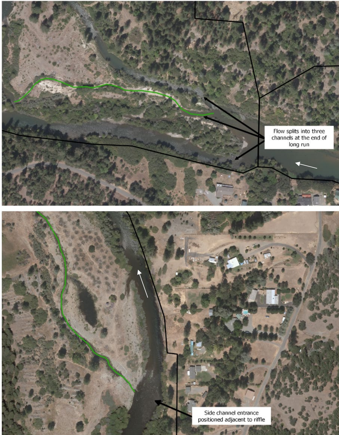
Figure 10. 2016 aerial photographs showing the geomorphic setting of side-channel R2 at Sawmill (top) and side-channel R4 at Lorenz Gulch (bottom). Both side-channels were constructed across wide floodplain areas and both have experienced deposition at the entrances. Deposition at Sawmill may have been greater because the flow splits into three channels, causing less flow and higher deposition in R3, and/or because the entrance is not positioned adjacent to or directly upstream of a riffle crest.
