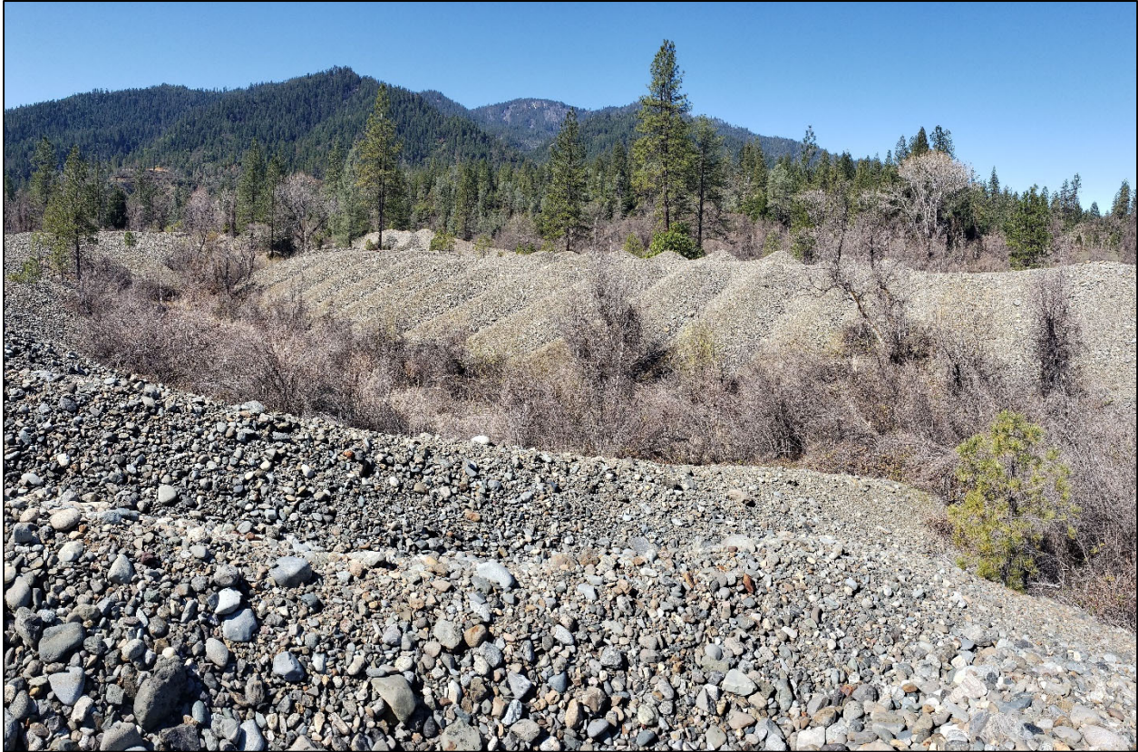
Figure 1. Mine tailings piles at the Oregon Gulch project site. Vegetation does not grow on the crests of the piles and is limited to low elevation areas between piles.
