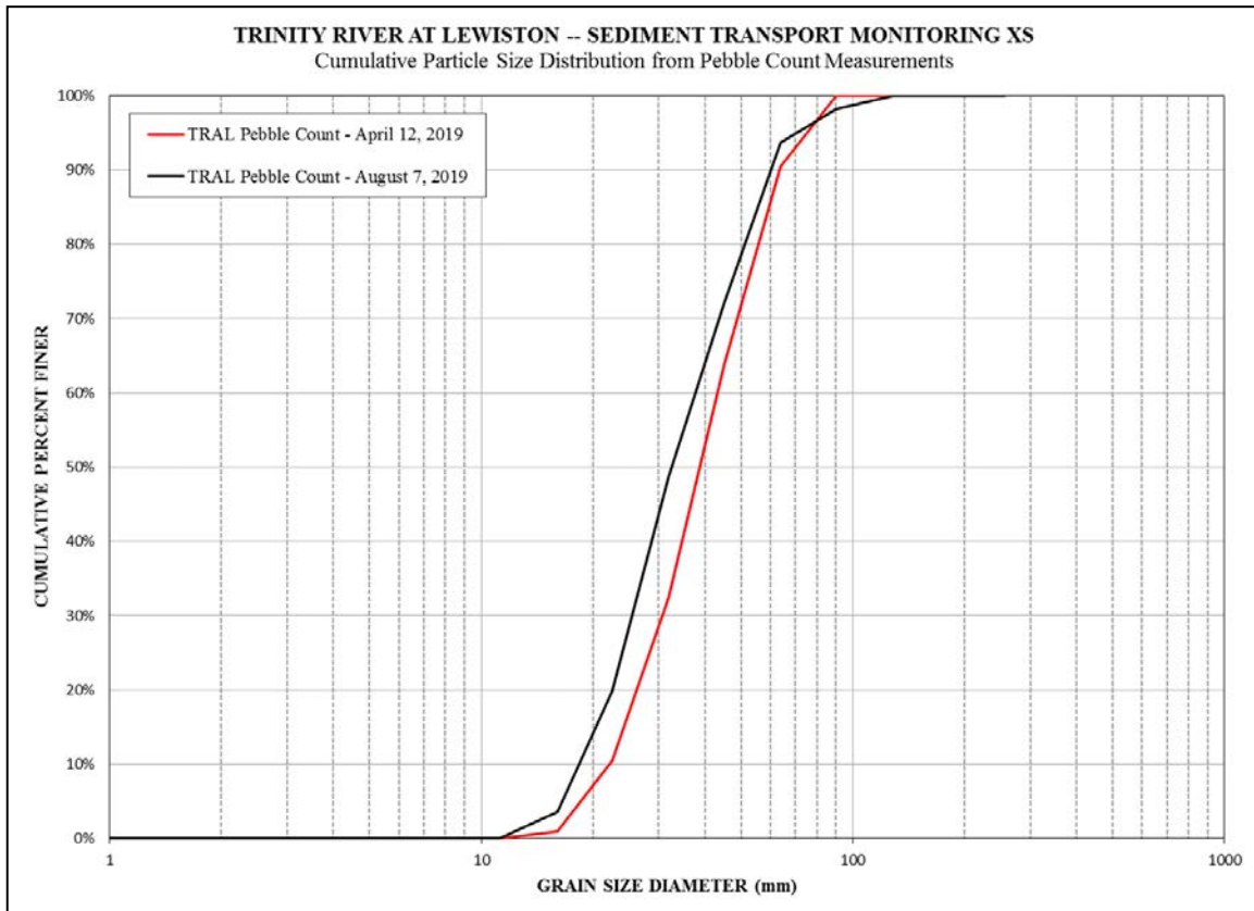
Figure 12. Changes in bed texture at TRAL, pre/post Spring Flow Release 2019.
