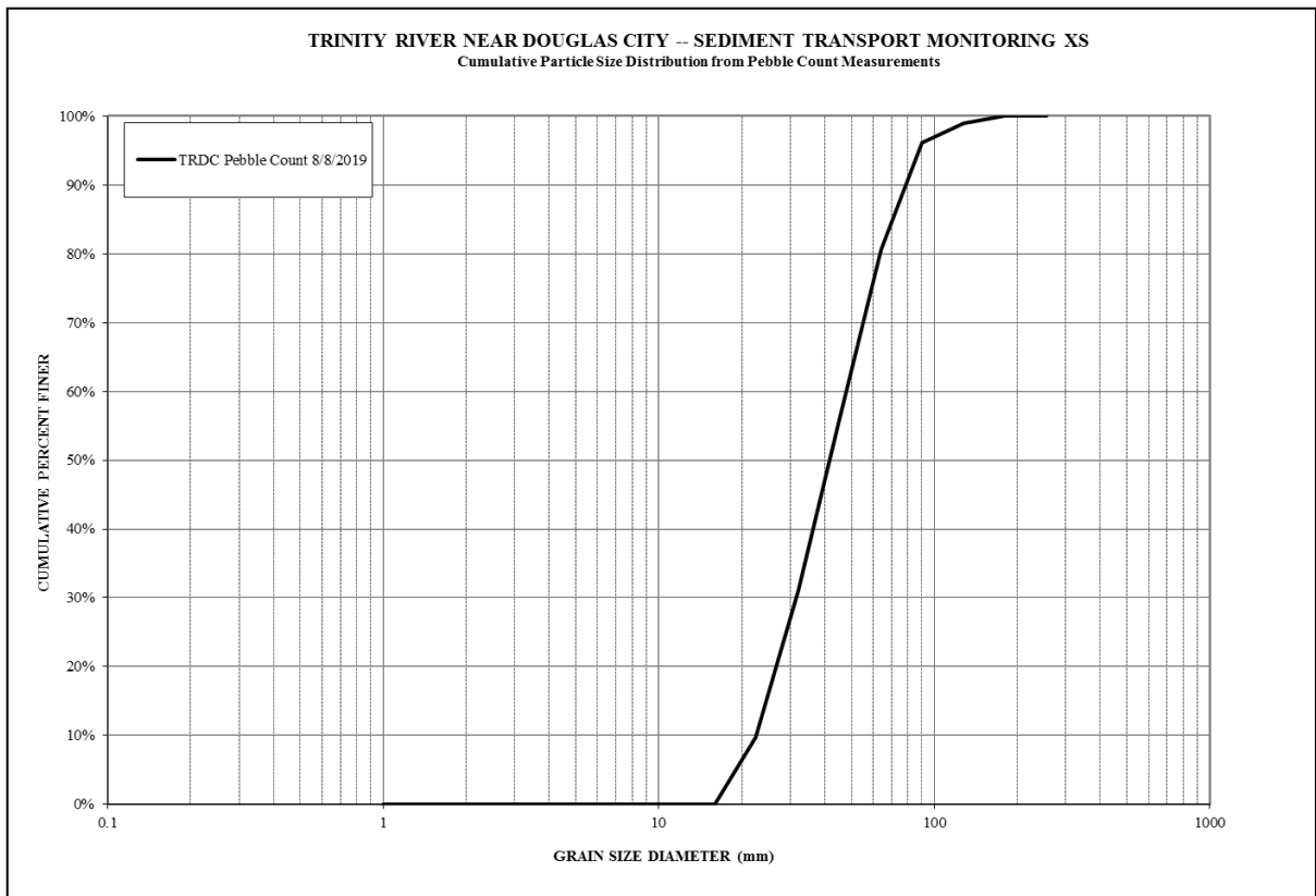
Figure 32. Changes in bed texture at TRDC, Spring Flow Release 2019.
