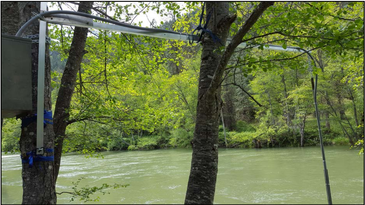
Figure 4. An articulating turbidity boom and gage house box deployed at TRGV in 2019.
