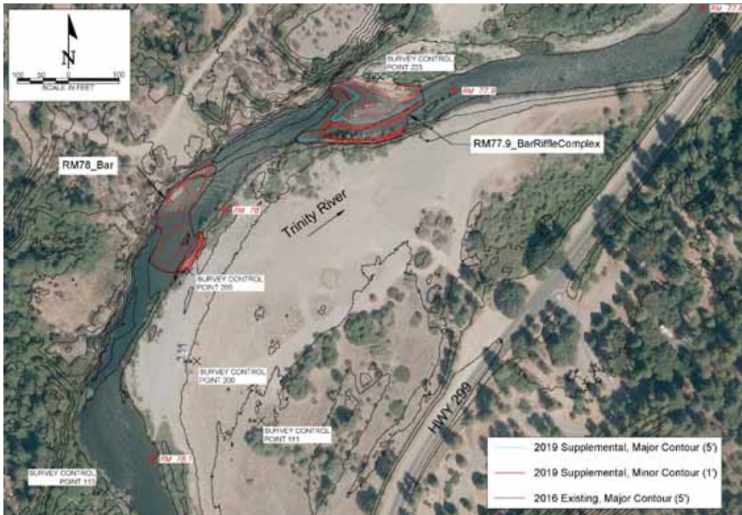
Figure 18. 2019 topographic supplemental survey for the evolved bar-riffle complexes at RM 77.9 and RM 78.0.
