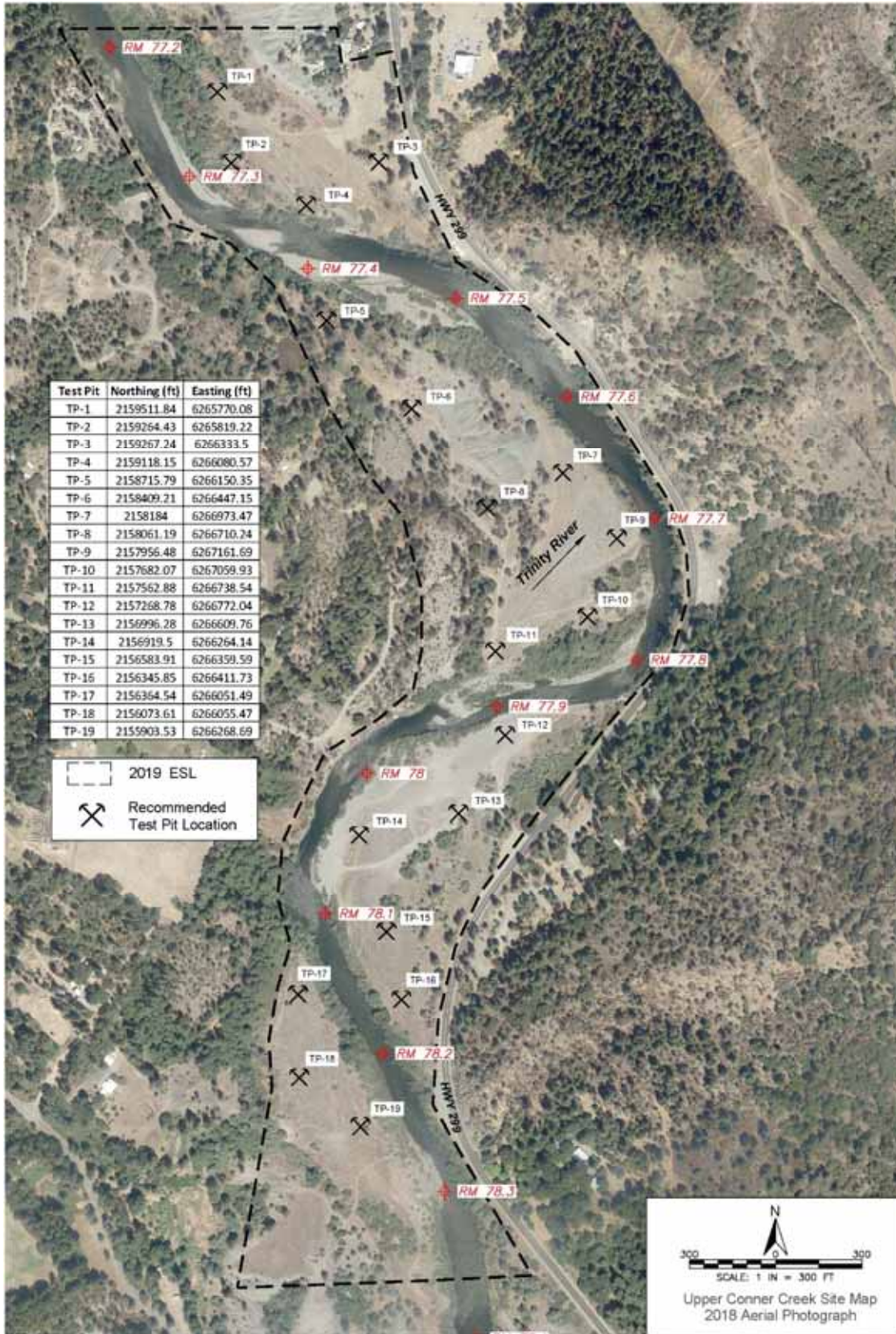
Figure 9. Recommended test pit locations.
