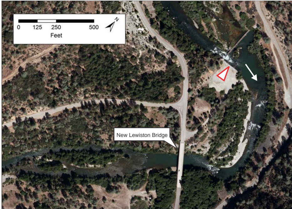
Figure 3: Aerial photograph of the Diversion Pool gravel injection location. The red triangle indicates the gravel injection point and the white arrow indicates flow direction.
