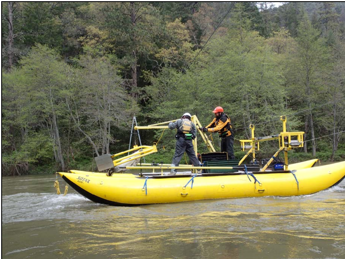
Figure 3. A 200 lb twin-tube TR2 bedload sampler deployed from a cataraft at the TRLG sampling site in April, 2017.
