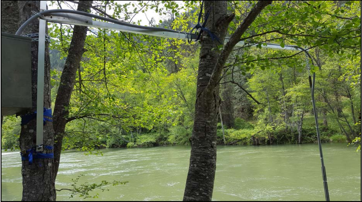
Figure 4. An articulating turbidity boom and gage house box deployed at TRGV in 2017.
