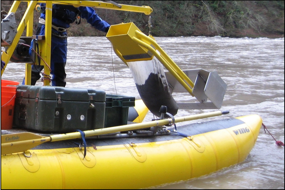
Figure 3. A 200 lb twin-tube TR2 bedload sampler deployed from a cataraft, Sandy River, OR.
