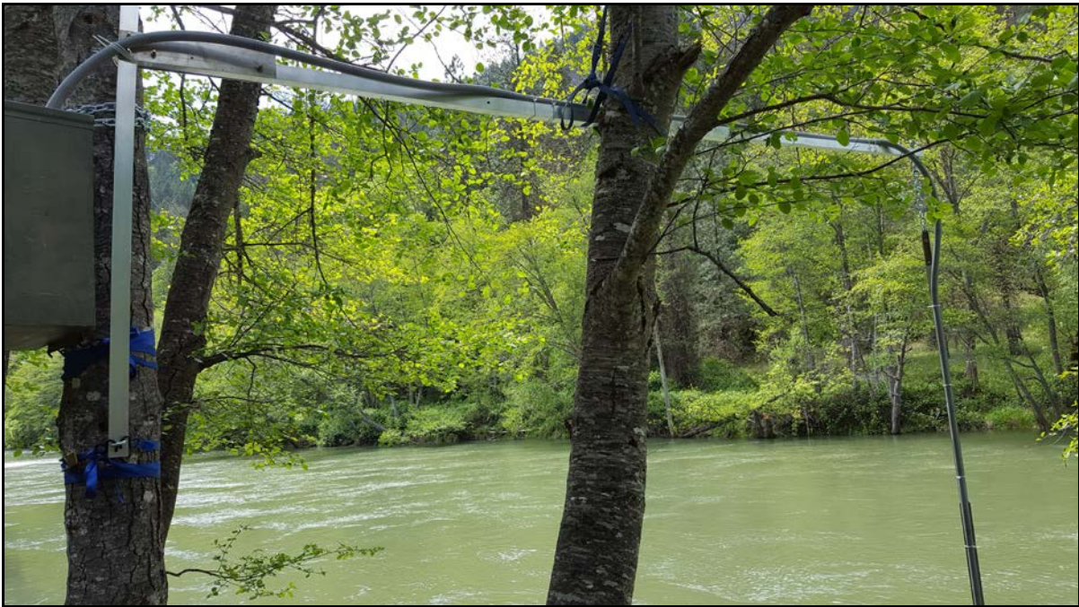
Figure 4. An articulating turbidity boom and gage house box deployed at TRGV in 2016.
