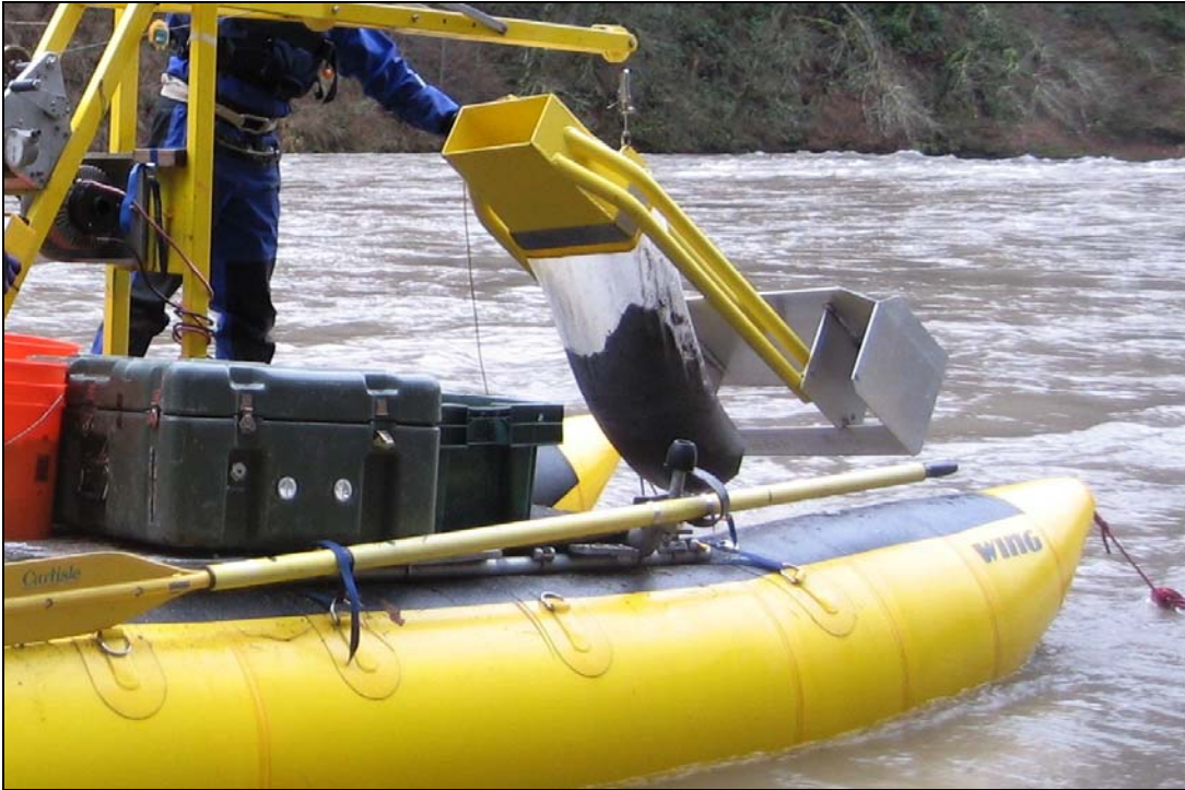
Figure 3. A 200 lb twin-tube TR2 bedload sampler deployed from a cataraft.
