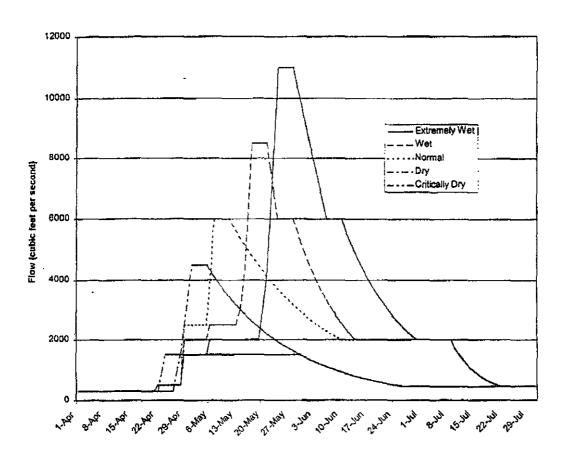
Figure 1. Proposed annual Trinity River hydrographs for each water year class: Extremely Wet, Wet, Normal, Dry, and Critically Dry. For all hydrographs, the proposed release from Lewiston Dam is 300 CFS from October 16 to April 8 and 450 CFS from August 1 to October 15. Data are from USFWS and HVT (1999).
